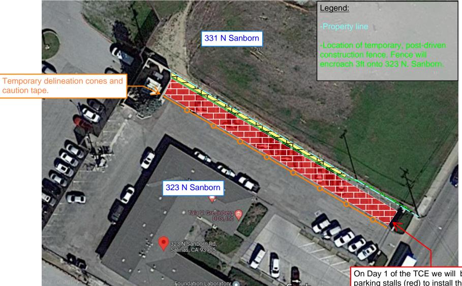
On Day 1 of the TCE we will block-off 20 parking stalls (red) to install the temporary construction fence (green). We will set up delineation cones and safety tape, as shown conceptually in orange. Duration of impact to parking lot will be 4 hours.
