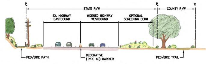
TYPICAL STATE ROUTE 68 WIDENING SECTION - NARROW CONFIGURATION
