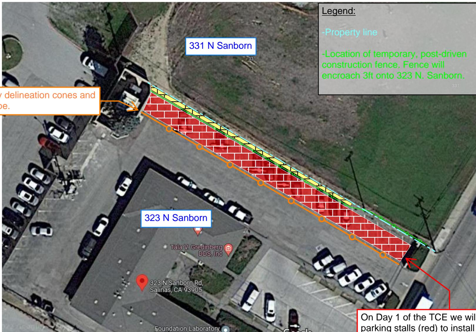
On Day 1 of the TCE we will block-off 20 parking stalls (red) to install the temporary construction fence (green). We will set up delineation cones and safety tape, as shown conceptually in orange. Duration of impact to parking lot will be 4 hours.
