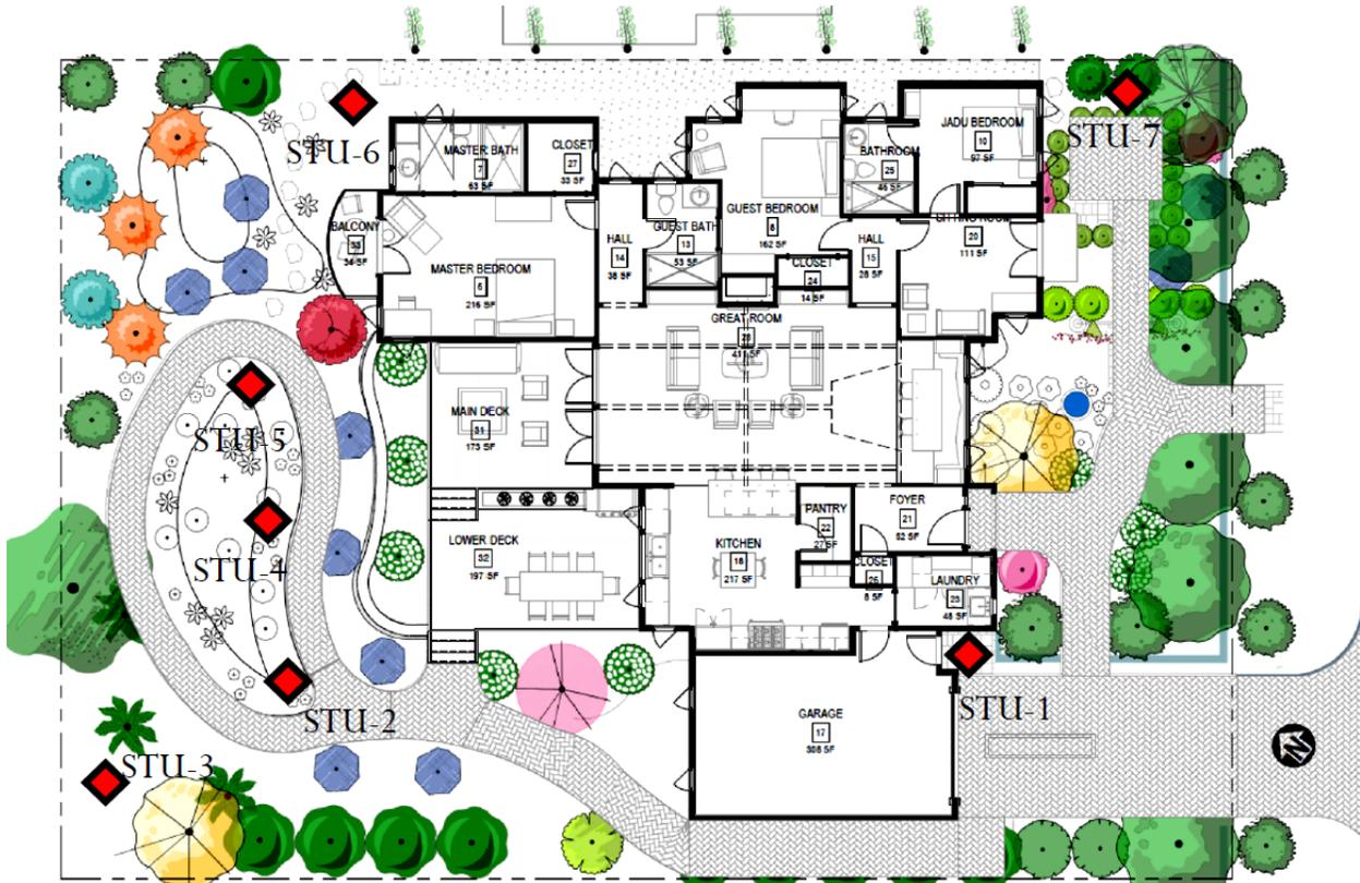
**Figure 7 Overlay of Proposed Residence on Existing Footprint & Locations of Geotechnical Bores (Source IX.38)**
