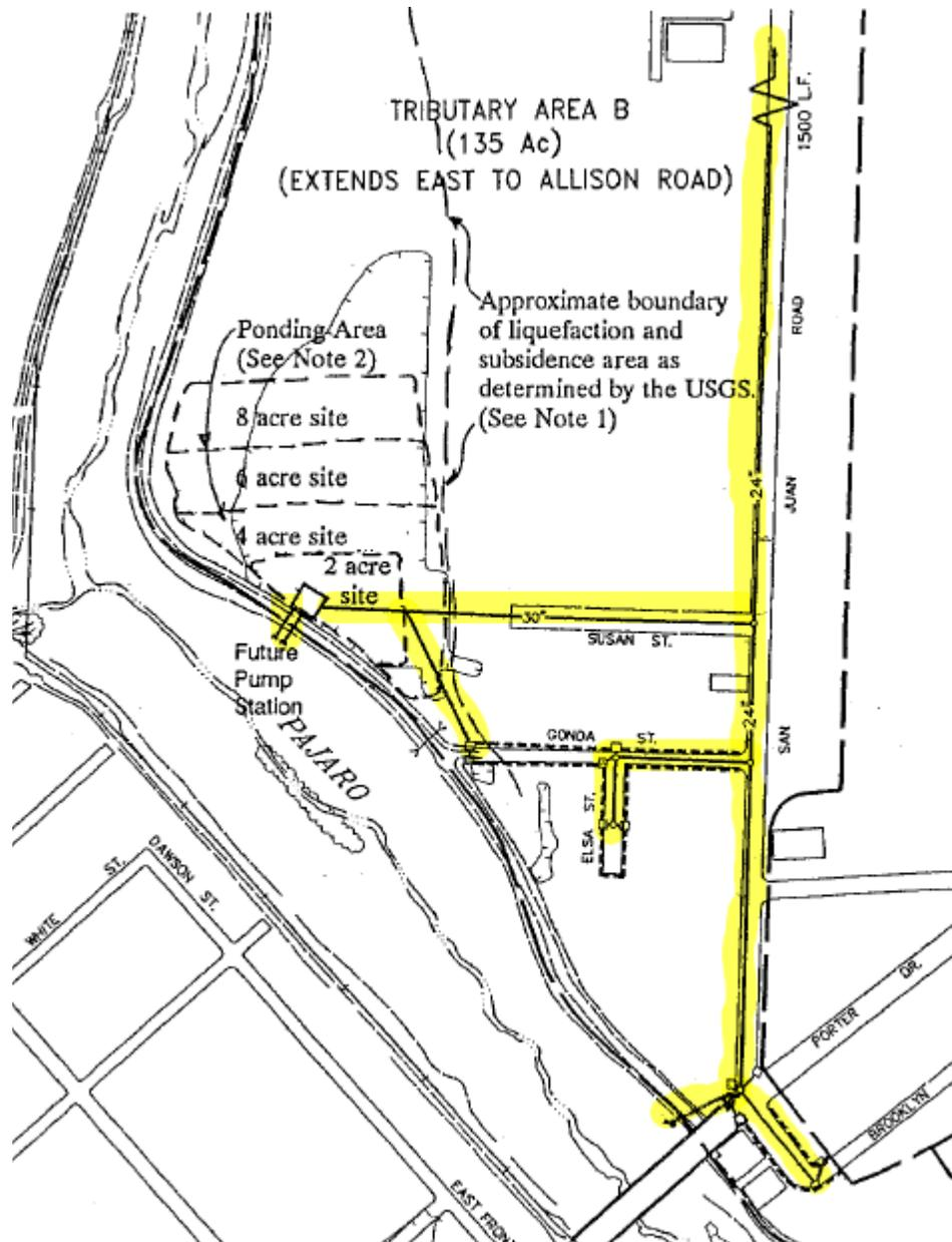
Figure 2. Excerpt from Figure 8, Pajaro Master Drainage Plan
