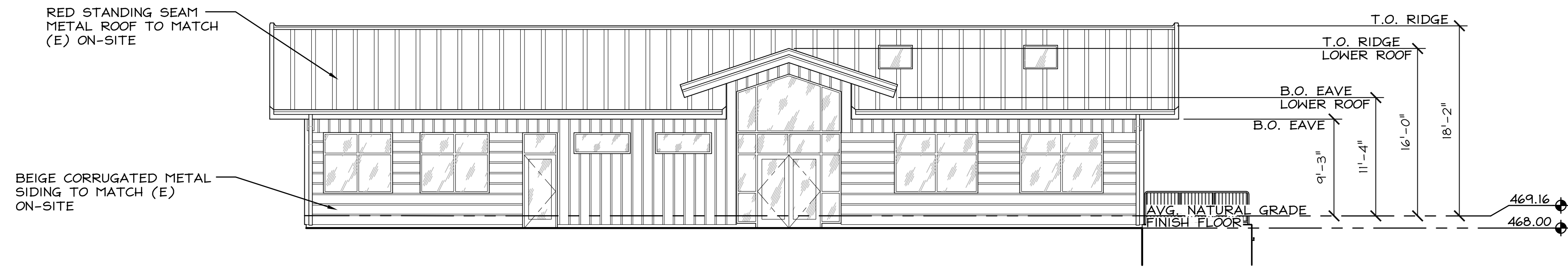
1 (N) TRAINING PAVILION - NORTH ELEVATION SCALE: 1/8" = 1'-0"
