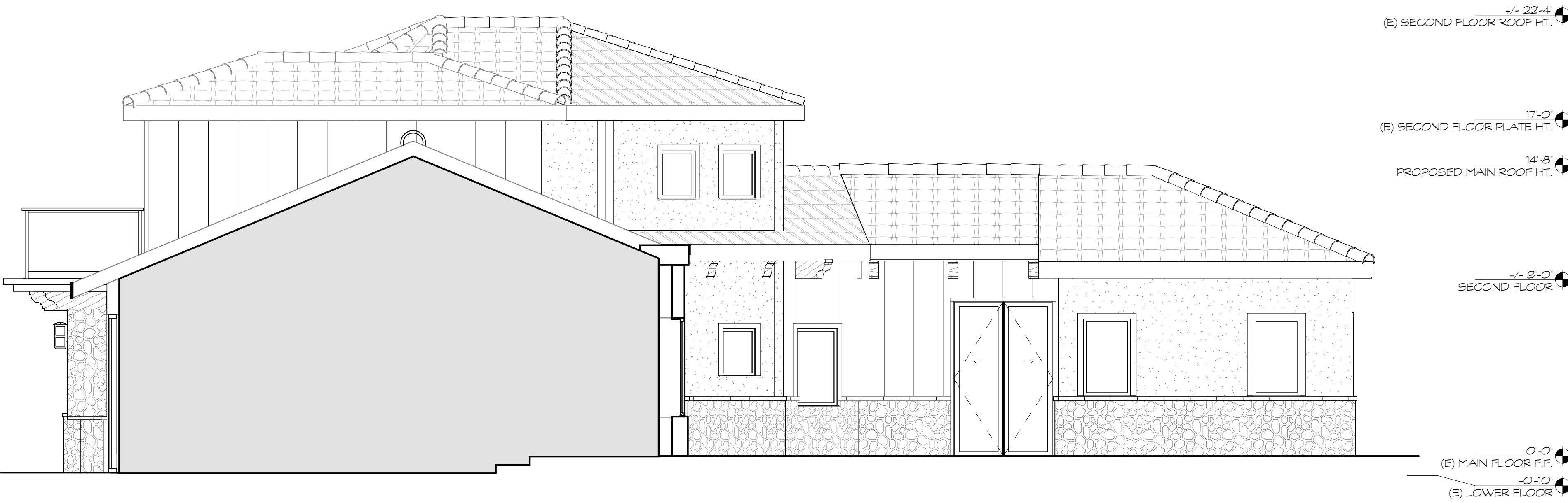
PROPOSED RESIDENCE - COURTYARD SOUTH ELEVATION/SECTION 2 1/4" = 1'-0"
