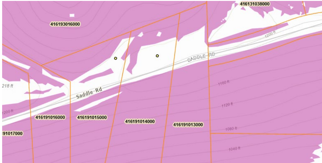
Figure 6: GIS information, all area shaded in pink is the approximate location of Slopes in excess of 25%.
