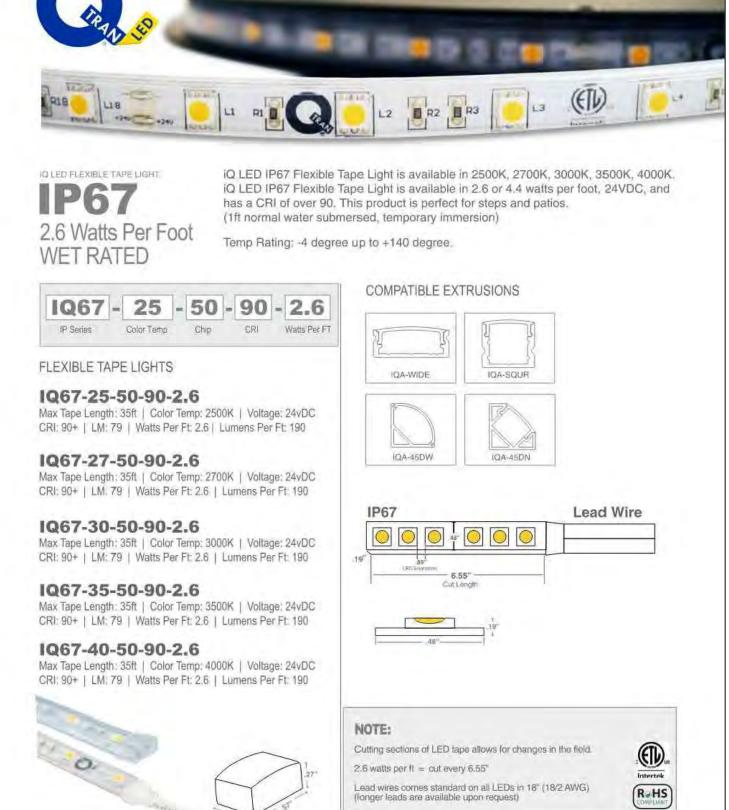
FIXTURE TYPE II: FLEXIBLE TAPE LIGHT AT STAIRS
