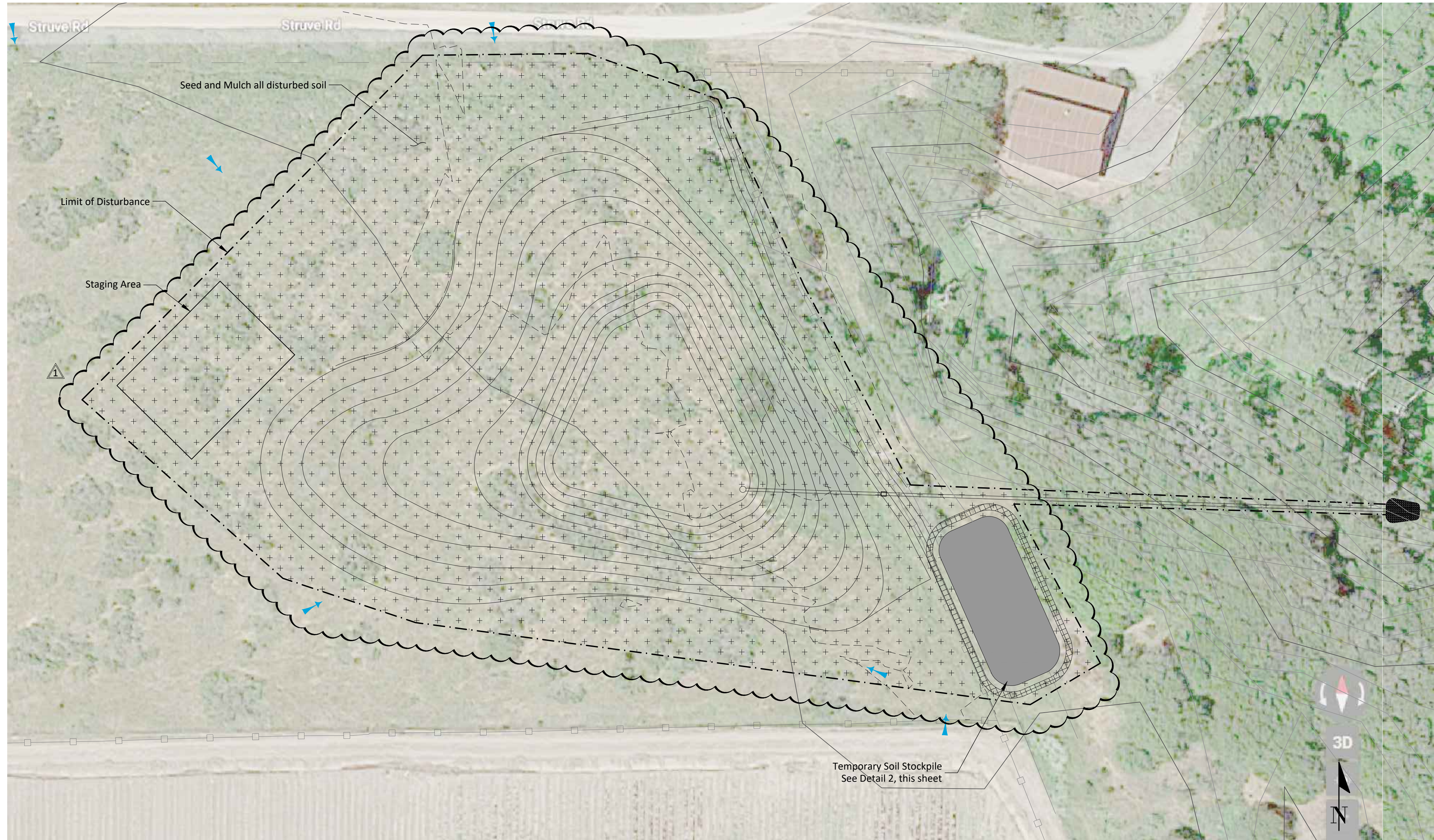
1 Erosion Control Layout Scale: 1" = 30'
