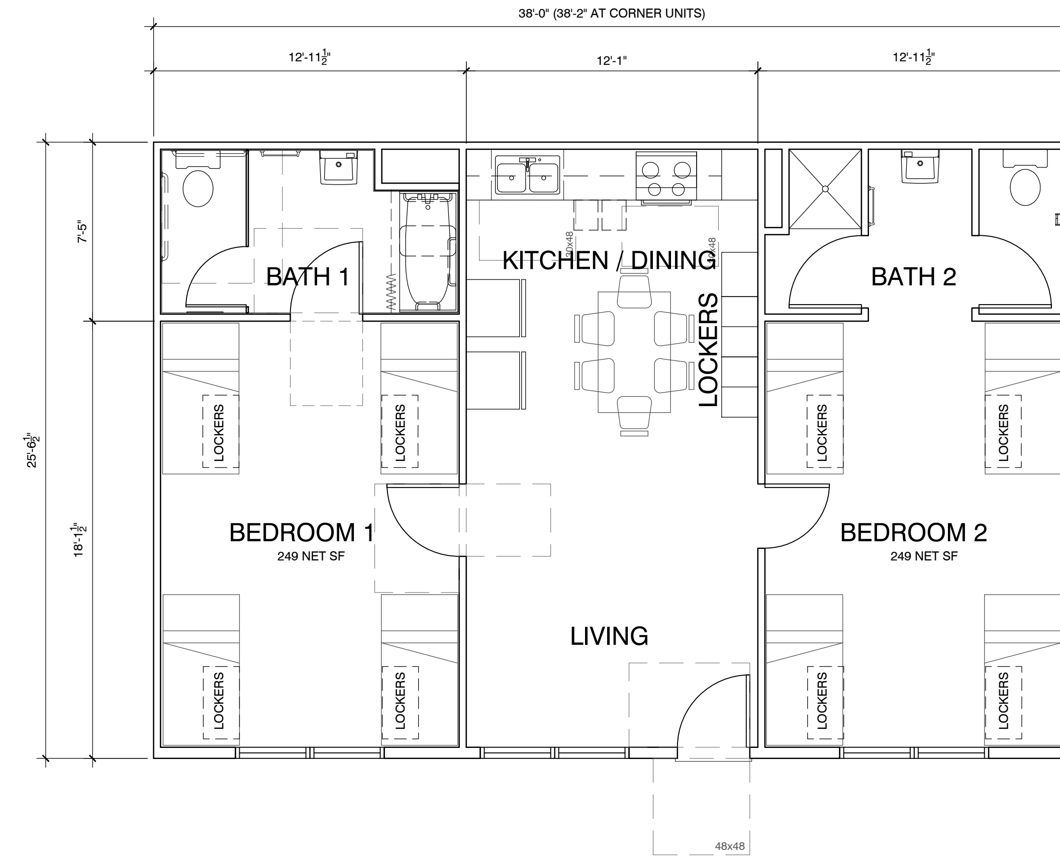
TYP. 1ST FLOOR UNIT PLAN
