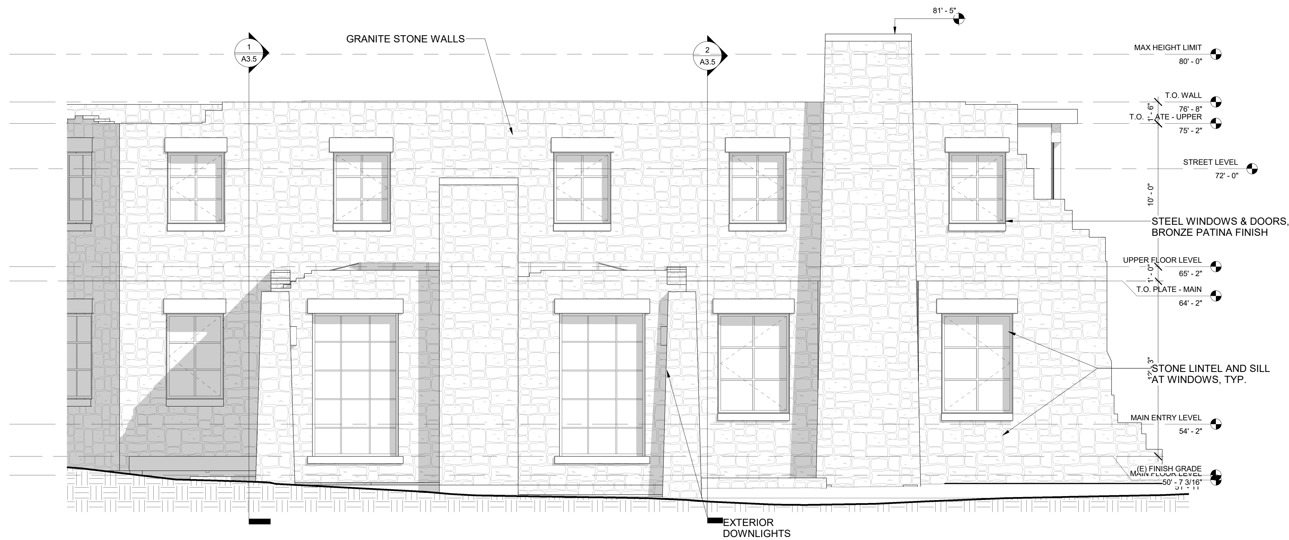
① WEST ELEVATION 1/4" = 1'-0"
