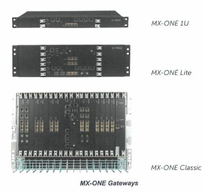
The MX-ONE 1U chassis is the choice for pure IP environments. There is also room for additional analog and a PRI connection. The MX-ONE 3U chassis, more suitable for IP environments and branch office scenarios with the space for up to five TDM boards. The MX-ONE Classic 7U chassis, fitted targets mainly mixed environments with space for up to 16 TDM legacy boards.
