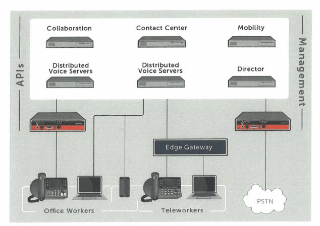
The Mitel Connect Edge Gateway improves access to the MiVoice Connect system for remote workers. With the Mitel Connect Edge Gateway, there is no need for off-site users to launch a VPN to use Mitel Connect IP phones.
