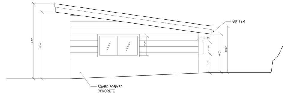
**4 GARAGE - S/E FACING EXTERIOR ELEVATION**
