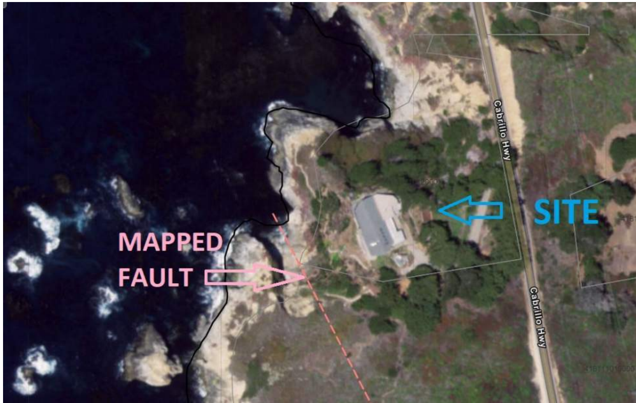
Figure 7: Close Up View of the Monterey County GIS Geologic Hazards Map Showing Mapped Fault Near Property
