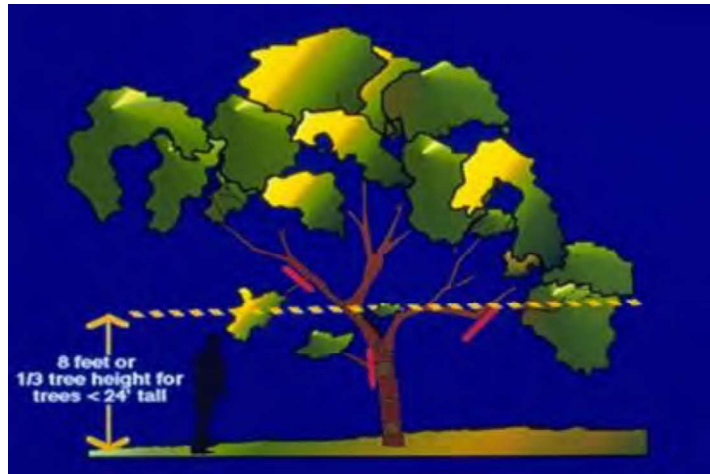
FIGURE 16 CREATE VERTICAL SPACING UNDER LOWER TREE BRANCHES BY REMOVING SMALL TREE BRANCHES FROM THE BOTTOM 8 FT OF THE TREE OR FROM THE BOTTOM ONE-THIRD OF THE TREE, WHICHEVER IS LESS.
