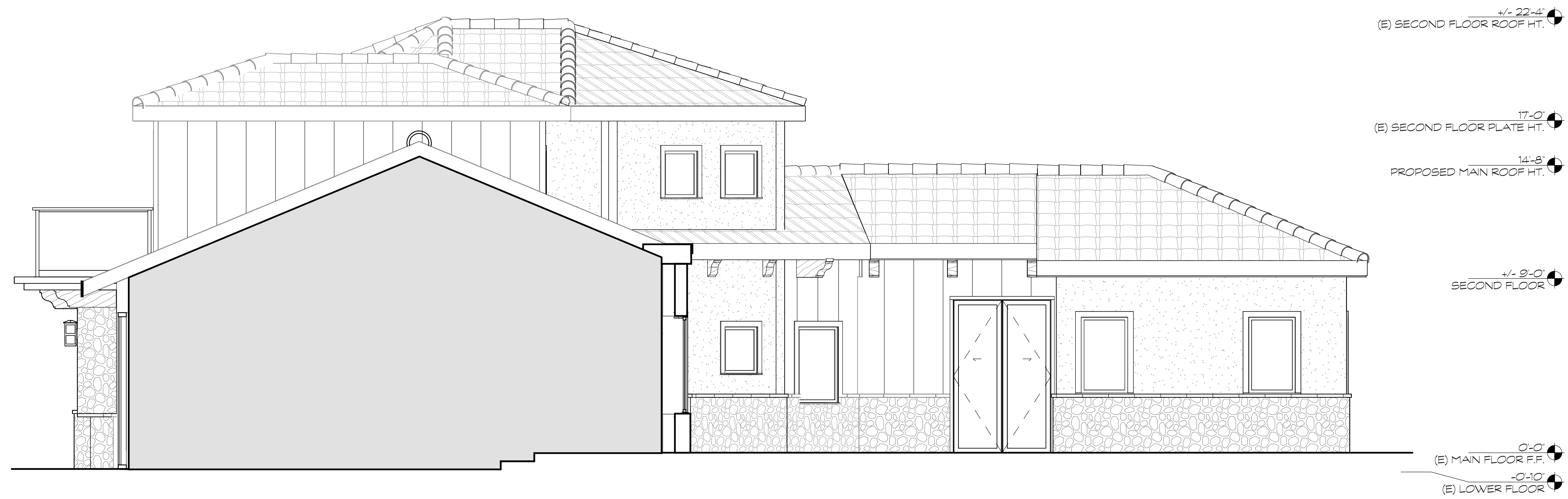
2 PROPOSED RESIDENCE - COURTYARD SOUTH ELEVATION/SECTION 1/4" = 1'-0"
