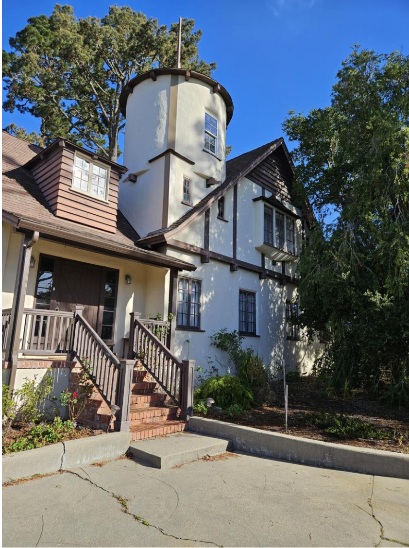
Figure 3: View of character-defining features on the front elevation, Including tower, half-timbering, oriel window, flared eaves, and Fenestration.
