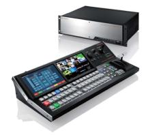
will reside in the Equipment Rack. The Controller simply connects with a single Ethernet Cable and sits on the Production Console.
