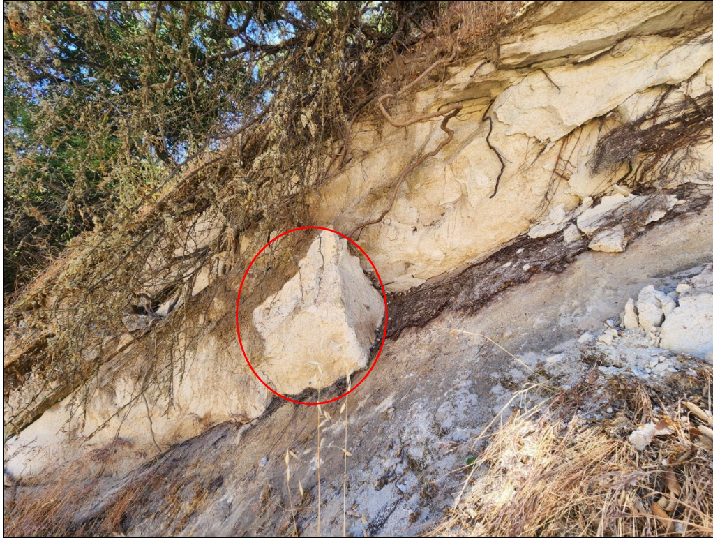
Photograph 2024-1. Close-up view of recent block failure location via planar sliding on bedding. Incipient block failure (approximately 1-foot in dimension) circled in red.
