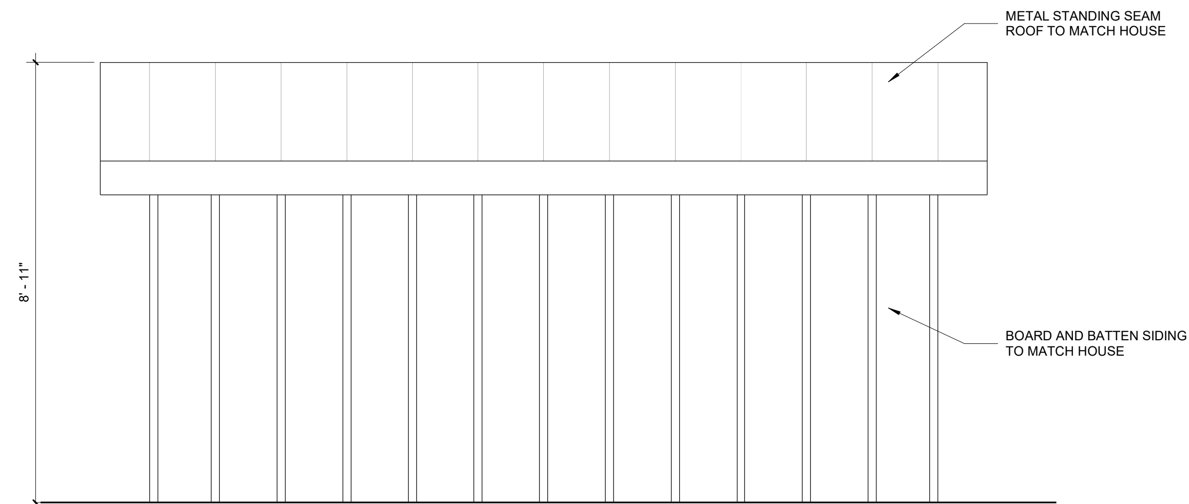
4 PUMP HOUSE - BUILDING ELEVATION - REAR 1/2" = 1'-0"
