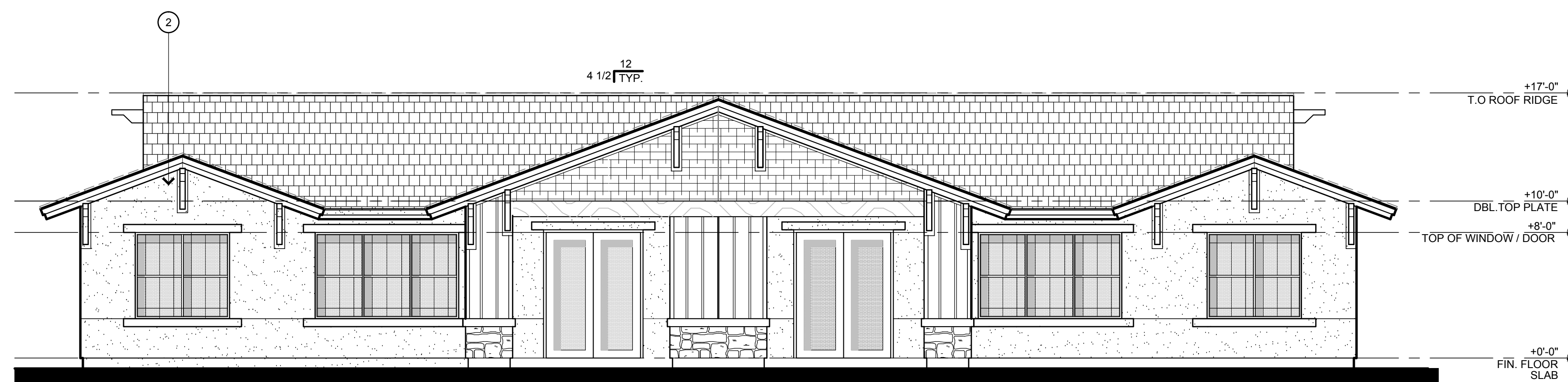
REAR ELEVATION - BUILDING TYPE 1 - A / A UNITS SCALE 3/16" = 1'-0" NOTE: MATERIALS ARE TYPICAL AT ALL ELEVATIONS AS SHOWN
