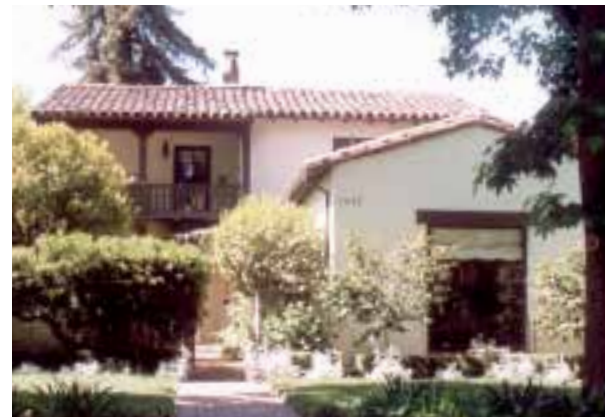
Many Mediterranean Revival houses possess a one-story projecting front wing to create a screened front yard.
