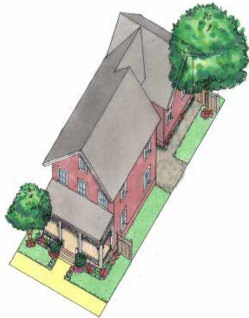
An East Garrison House Simple, dignified massing with porches and rear wings added.
