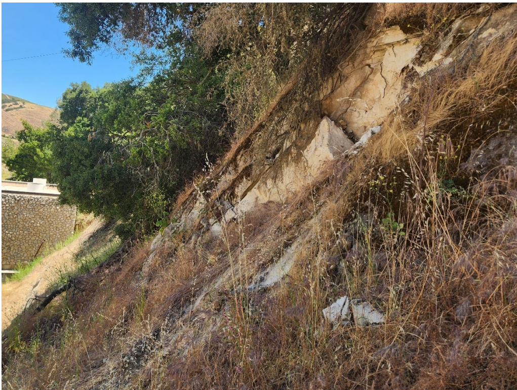
2024 Photograph 7. Small (1 foot in dimension) block failure since 2019. Failure occurred via planar sliding along bedding. Trees appear to be leaning down slope slightly more than observed in 2019.
