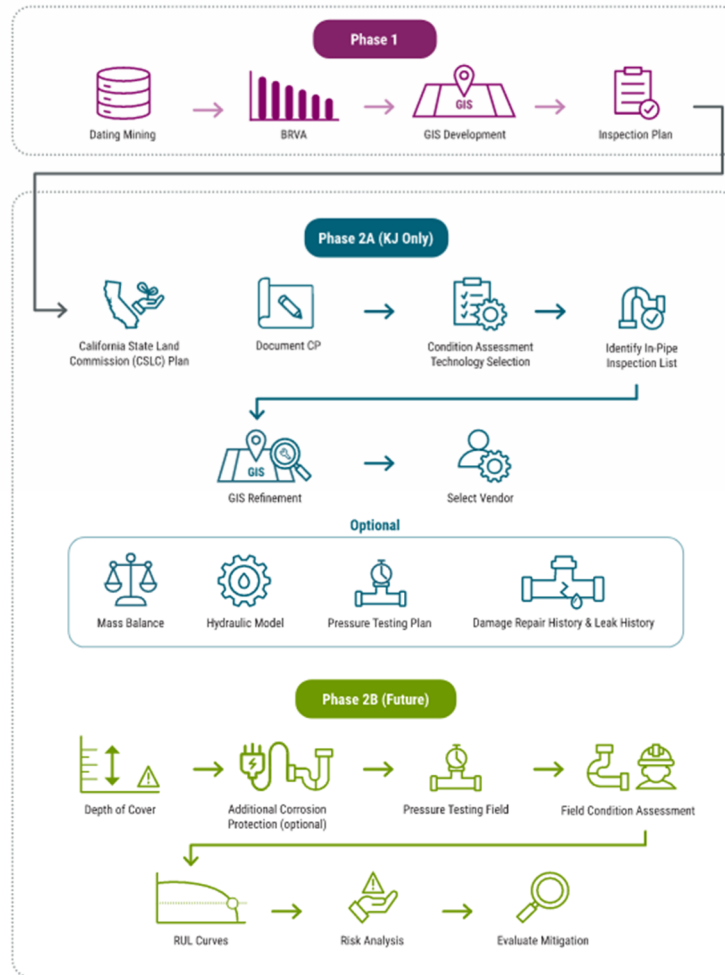
Figure 2. Phase 1 of Risk-Based Condition Assessment and Asset Management Process for CSIP with Progression to Phase 2A (in this proposal) and 2B (future).
