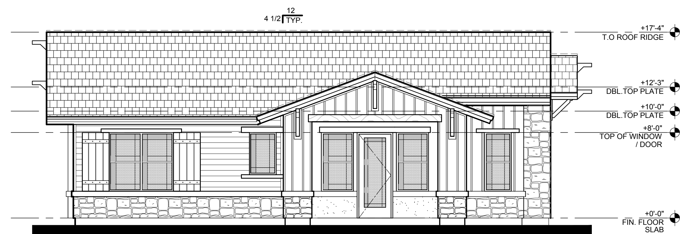
REAR ELEVATION - BUILDING TYPE 51 - B UNITS
