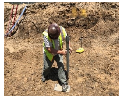
Sonic testing of trench back-fill.
