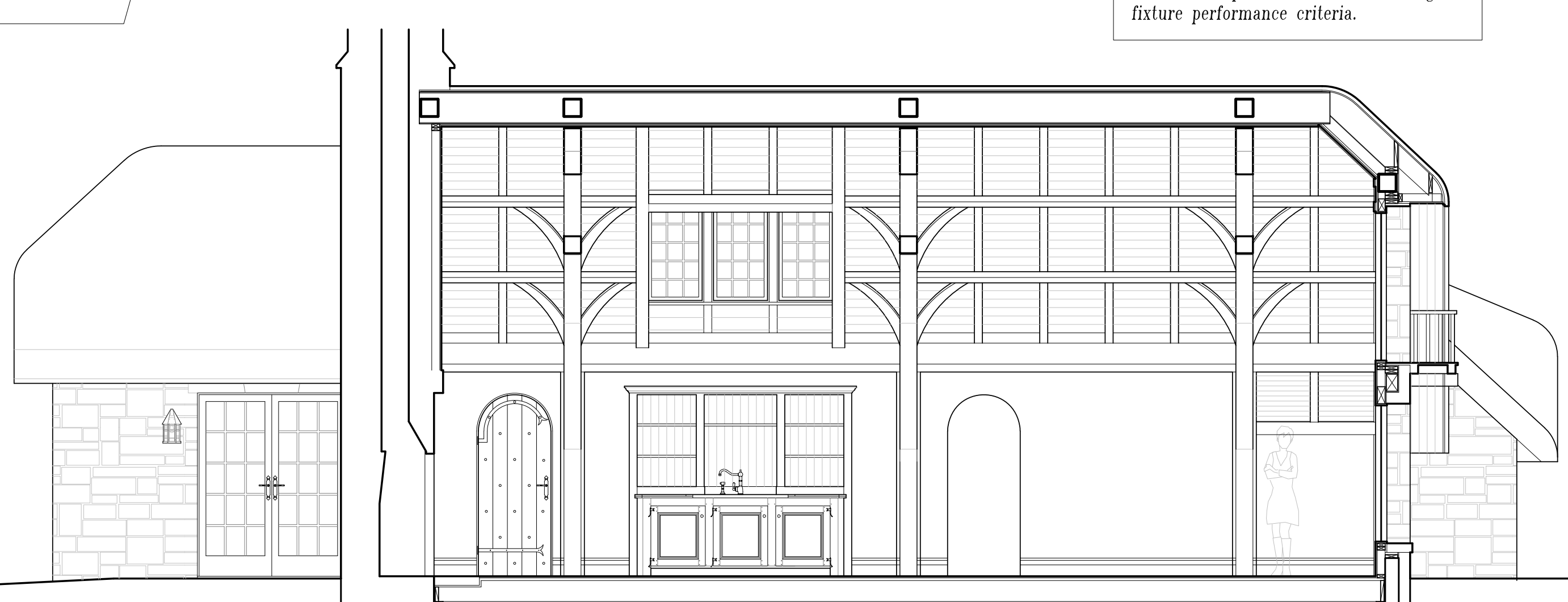
3 Section at Living room facing west - Lot A Scale: 1/4" = 1'-0"
