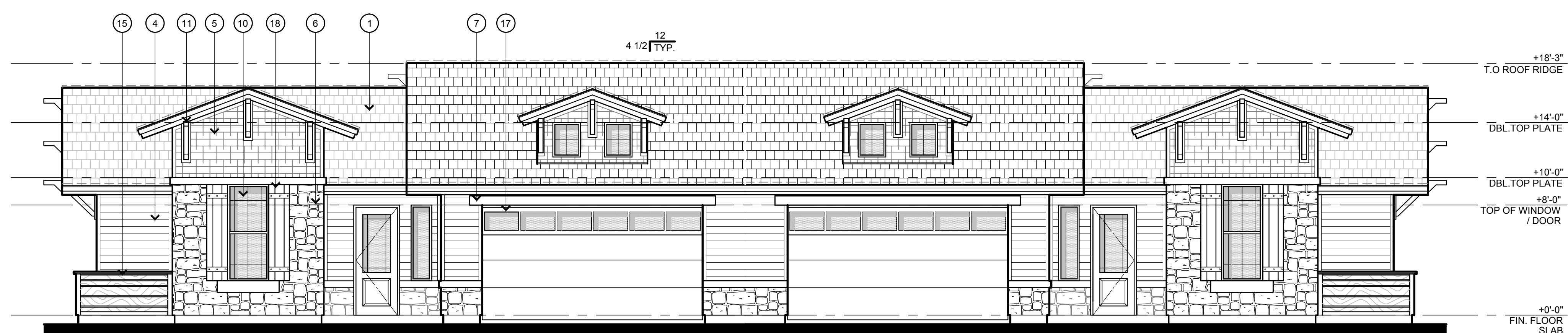
FRONT ELEVATION - BUILDING TYPE 4 - C / C UNITS SCALE 3/16" = 1'-0" NOTE: MATERIALS ARE TYPICAL AT ALL ELEVATIONS AS SHOWN
