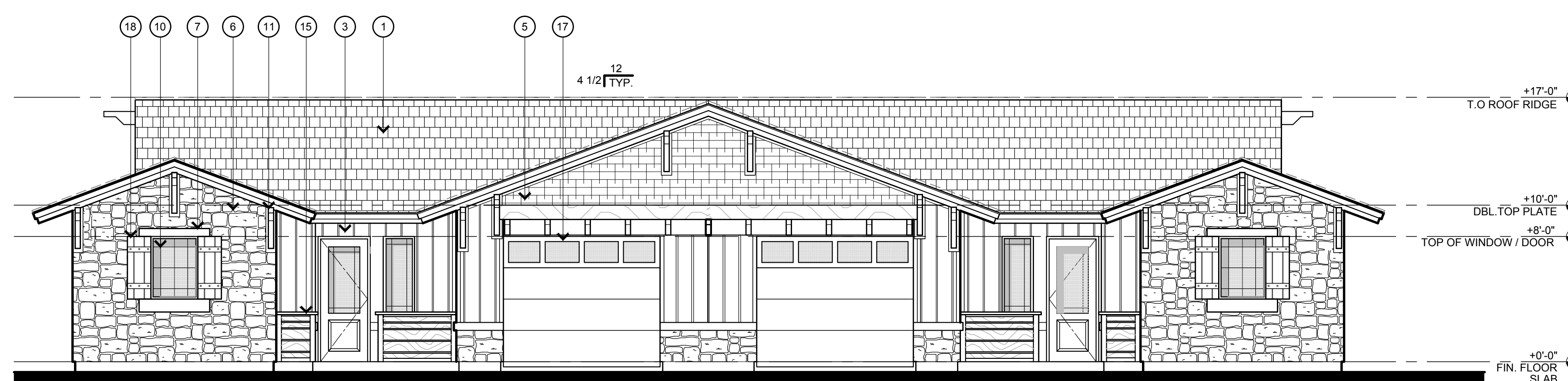
FRONT ELEVATION - BUILDING TYPE 1 - A / A UNITS SCALE 3/16" = 1'-0" NOTE: MATERIALS ARE TYPICAL AT ALL ELEVATIONS AS SHOWN
