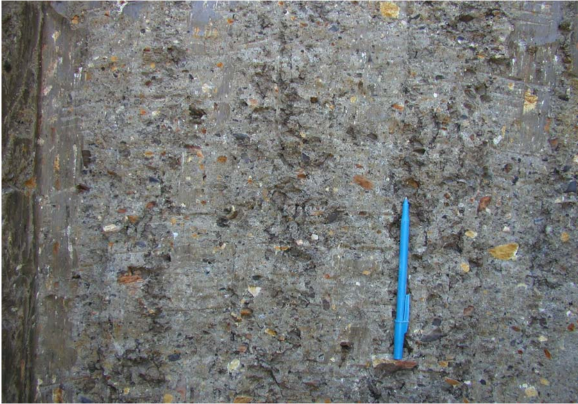
Photograph No. 12: Test pit 4, Lot 4. Lean clay with abundant siltstone and porcelanite fragments.
