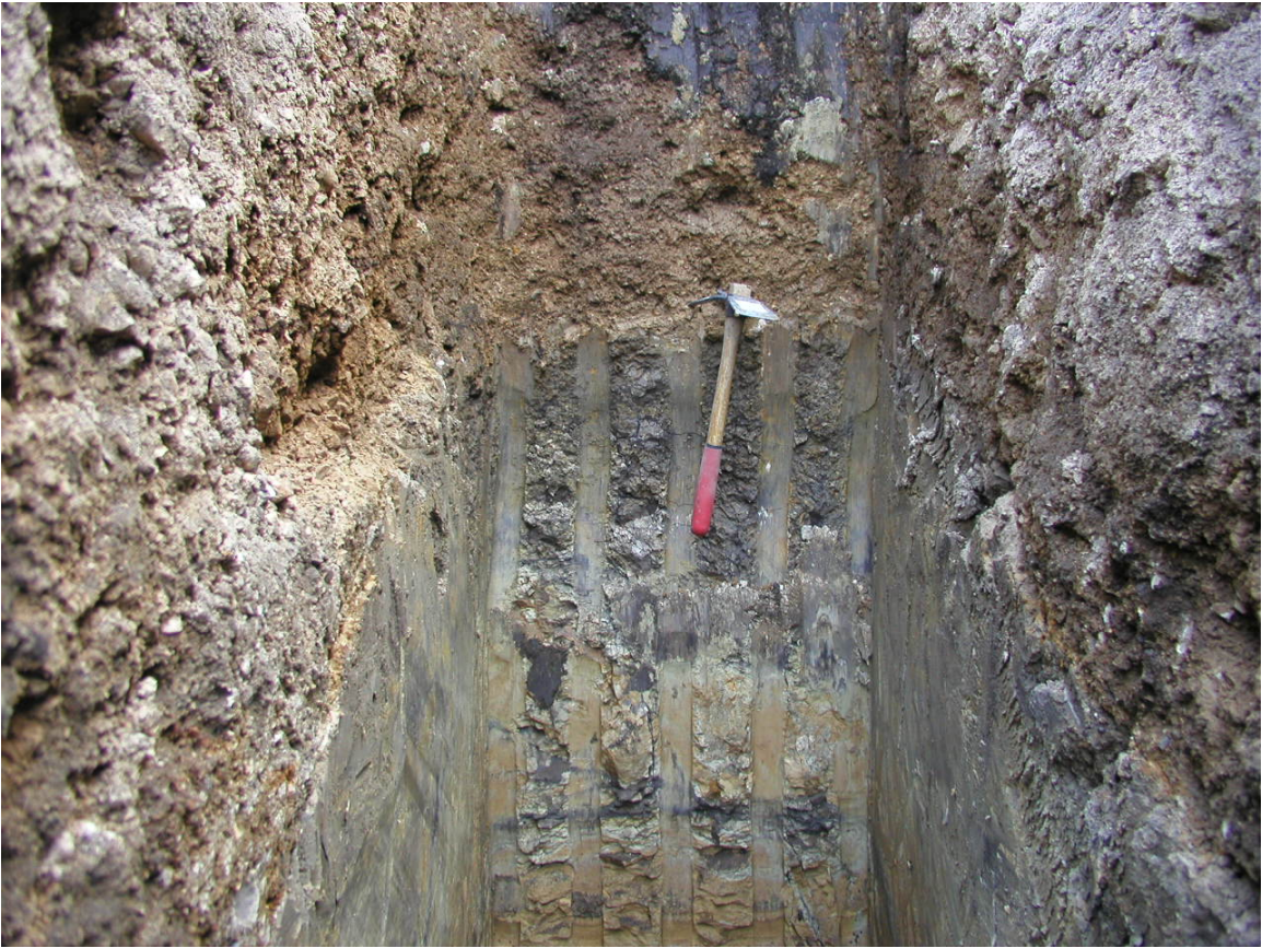
Photograph No. 9: Test pit TP-1, Lot 5. Pick head at bottom of grayish tan slit with abundant siltstone and porcelanite fragments. Silt is underlain by lean clay with siltstone and porcelanite fragments and intensely fractured and sheared siltstone below the pick handle.
