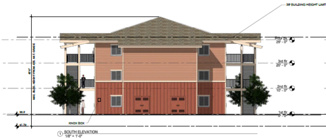
Figure 4b. South elevation for both buildings is shown above. The measurement on the left shows the building height is proposed as 43 feet above natural grade.
