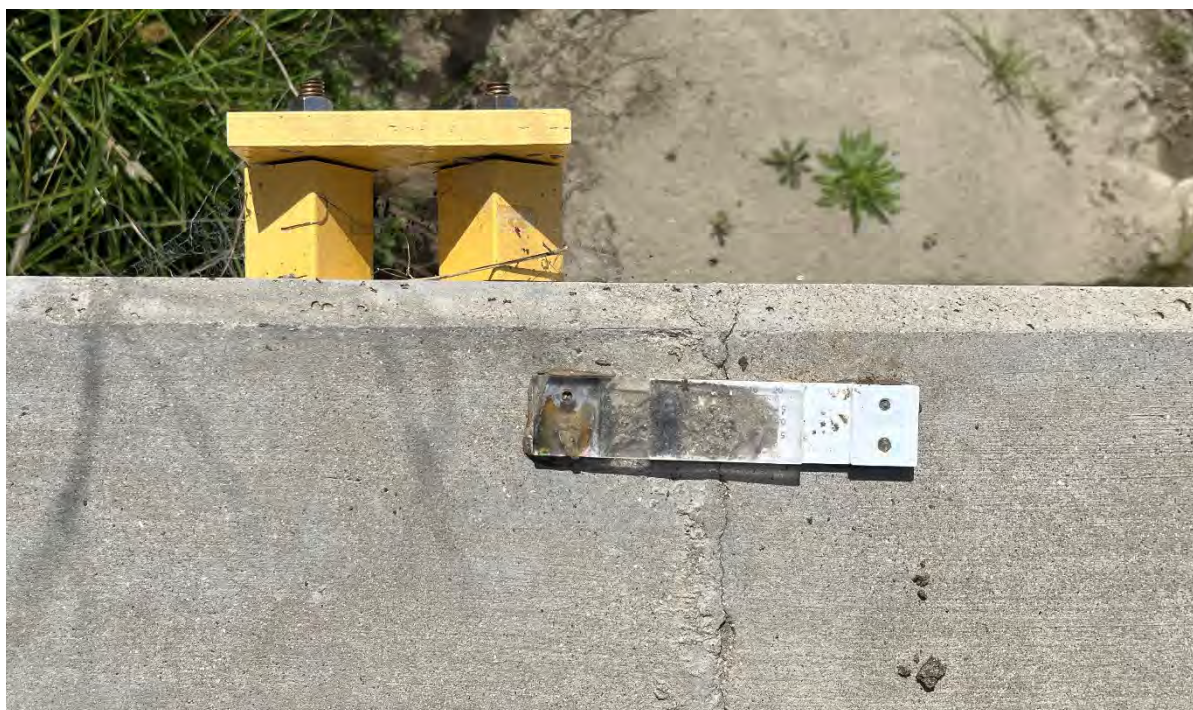
Figure 3: Crack Meter needs cleaning.
