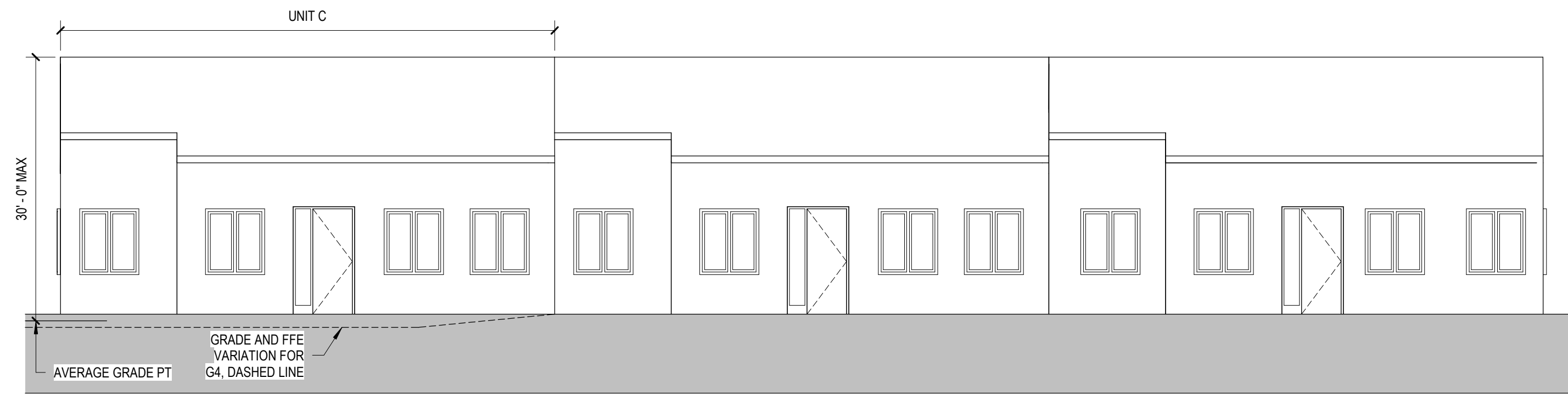
5 OFFSITE DUPLEX - NORTH ELEVATION (G2 & G4) 1/8" = 1'-0"
