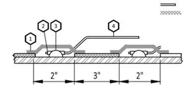
**DETAIL 3** ATTACHING THE WIRES TO THE GAS MAIN
