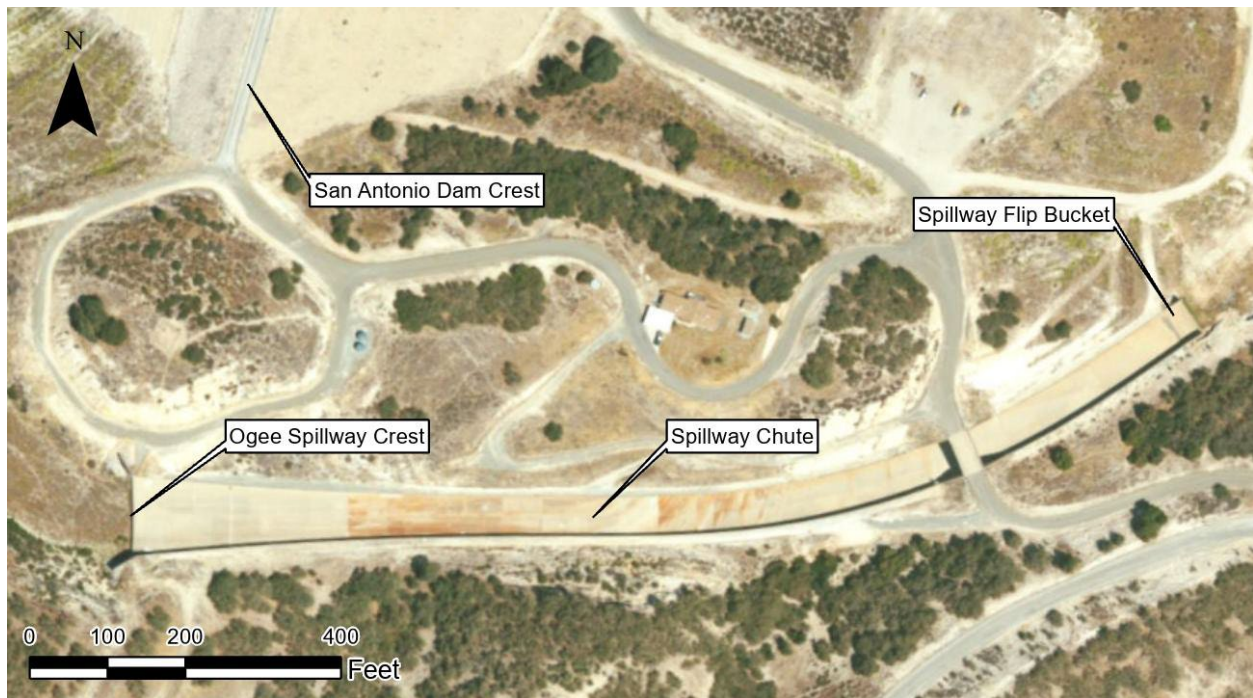
Figure 2: San Antonio Dam Spillway Alignment
