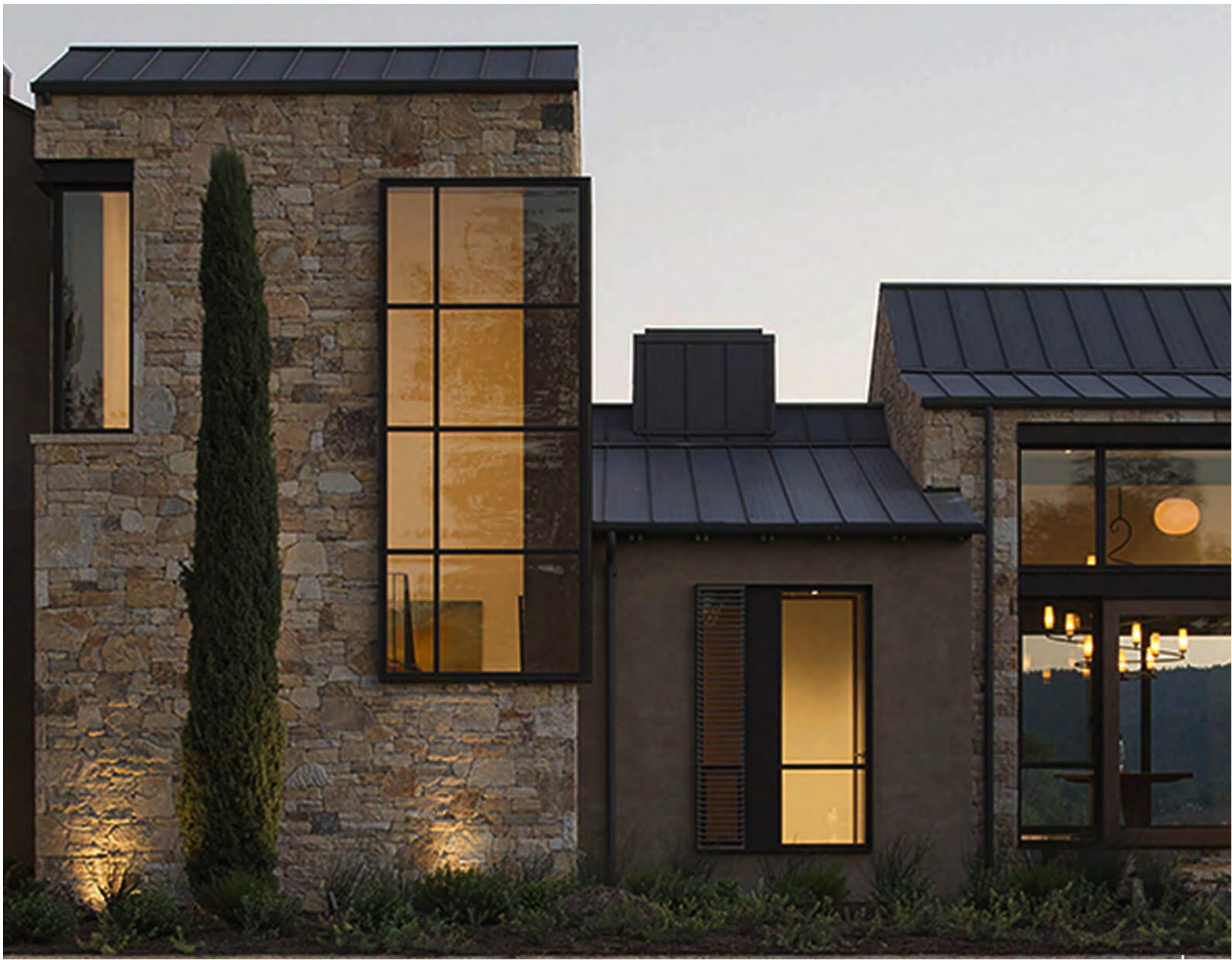
WINDOW & DOORS: JADA THERMALLY BROKEN STEEL DOORS AND WINDOWS; FINISH: TBD (DARK)
