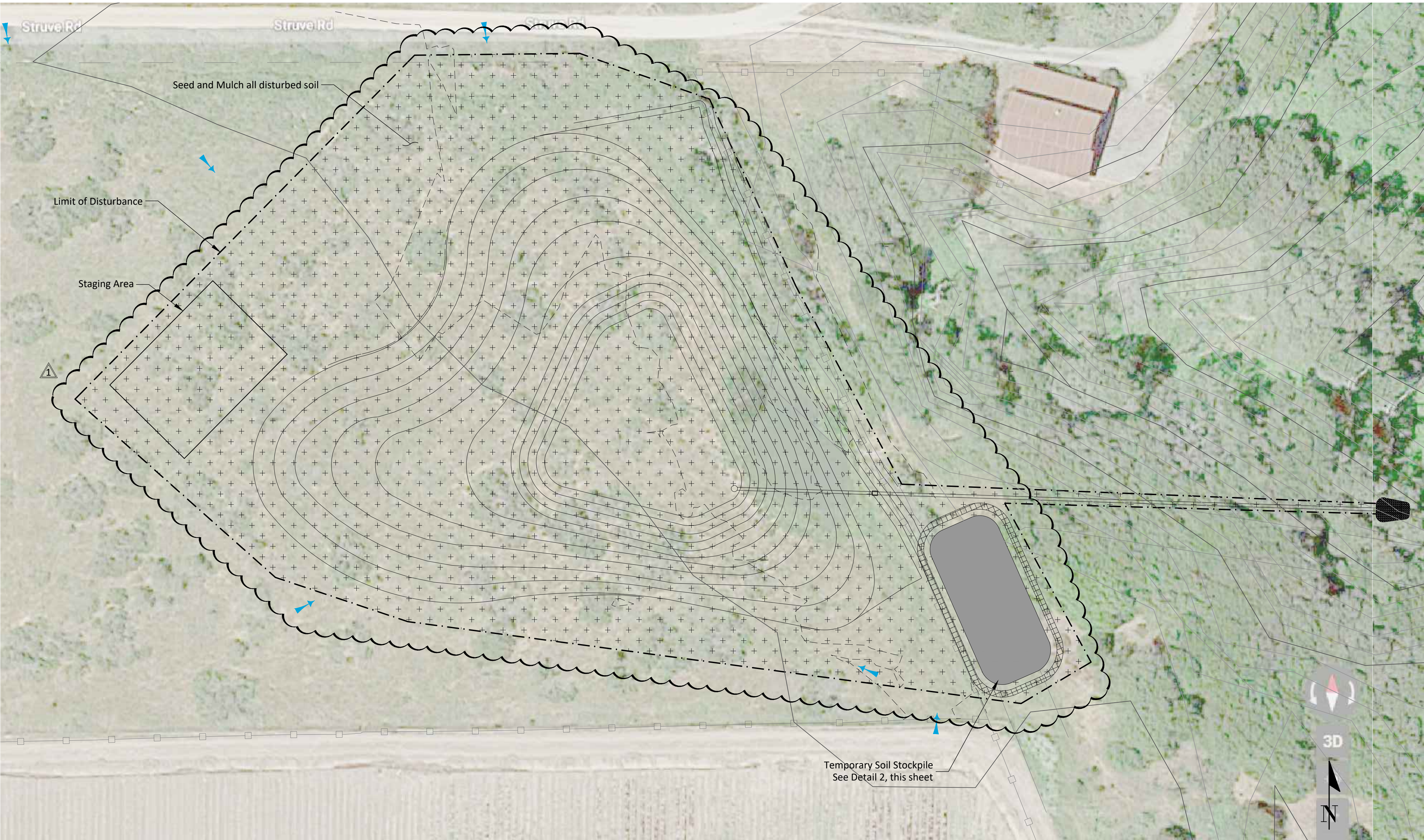
1 Erosion Control Layout Scale: 1" = 30'
