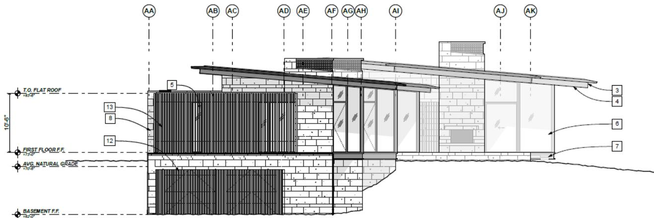
**Figure 1e – Proposed Exterior Elevations:** The north and west elevations, respectively. The existing structure is outlined in red. (Source IX.1)
