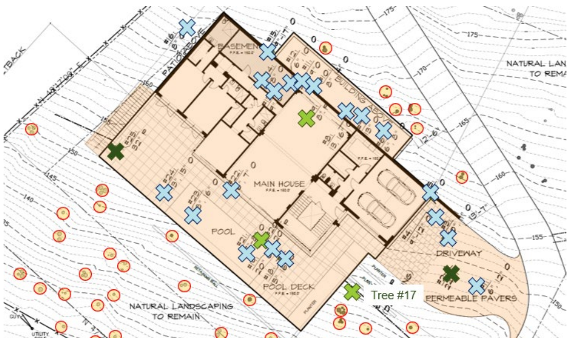
Figure 7: February 14, 2024 site plan, with trees proposed for removal shown as “X’s”. Oaks are blue while pine are green, and the landmark Monterey pine are darker green
