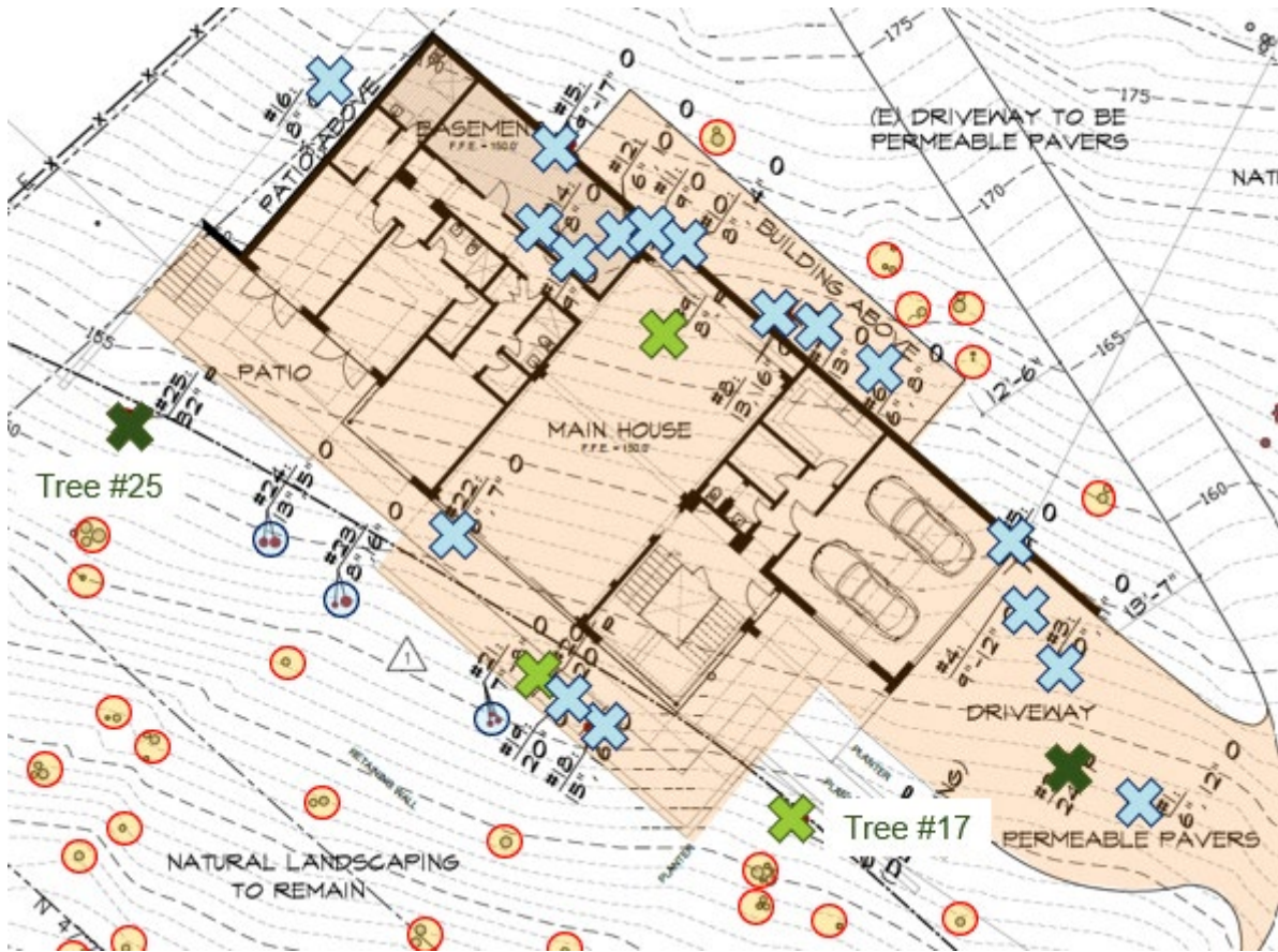
Figure 8: Revised site plan, with trees proposed for removal shown as “X’s”. Oaks are blue while pine are green, and the landmark Monterey pine are darker green. Trees that will be retained from this revised design, Coast Live oak #21, #23, and #24, are circled in blue
