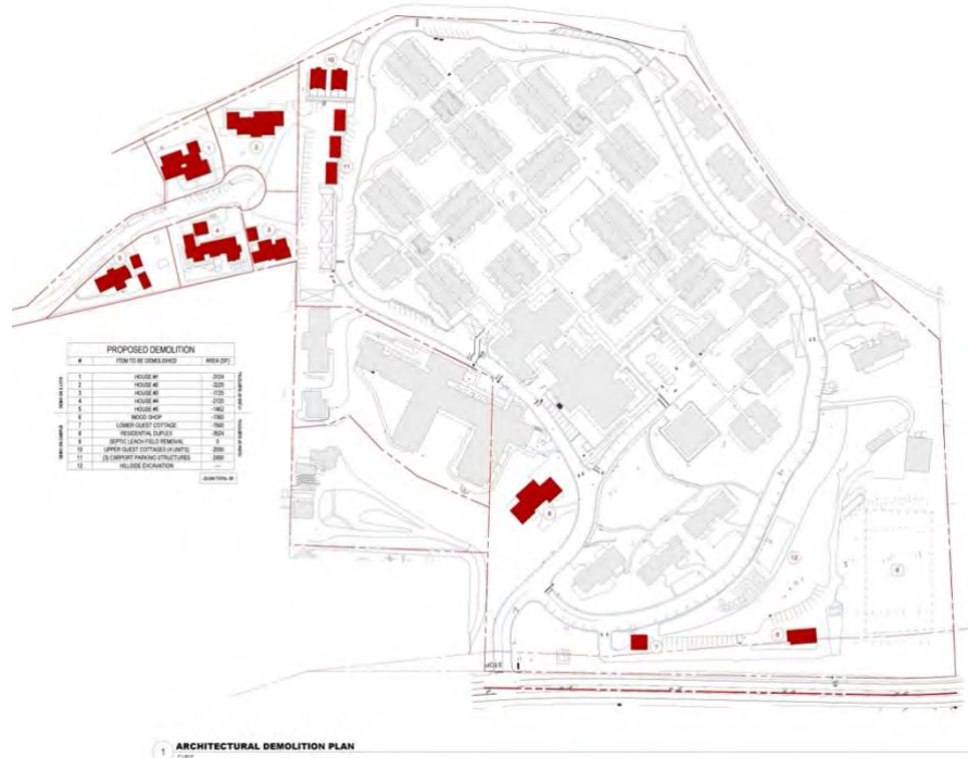
Figure 3. Site Plan showing buildings to be removed in red (Courtesy: Perkins Eastman, 2025).
