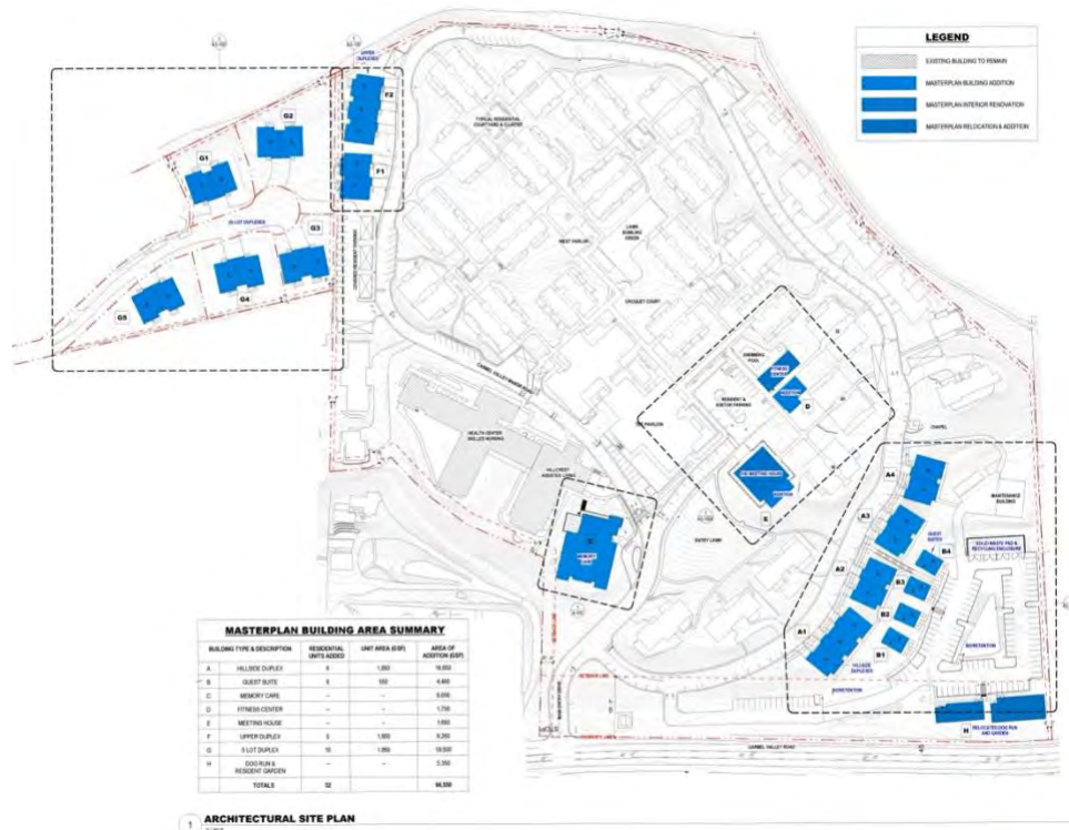
Figure 4. Site Plan showing buildings to be constructed in blue ( Courtesy: Perkins Eastman, 2025 ).
