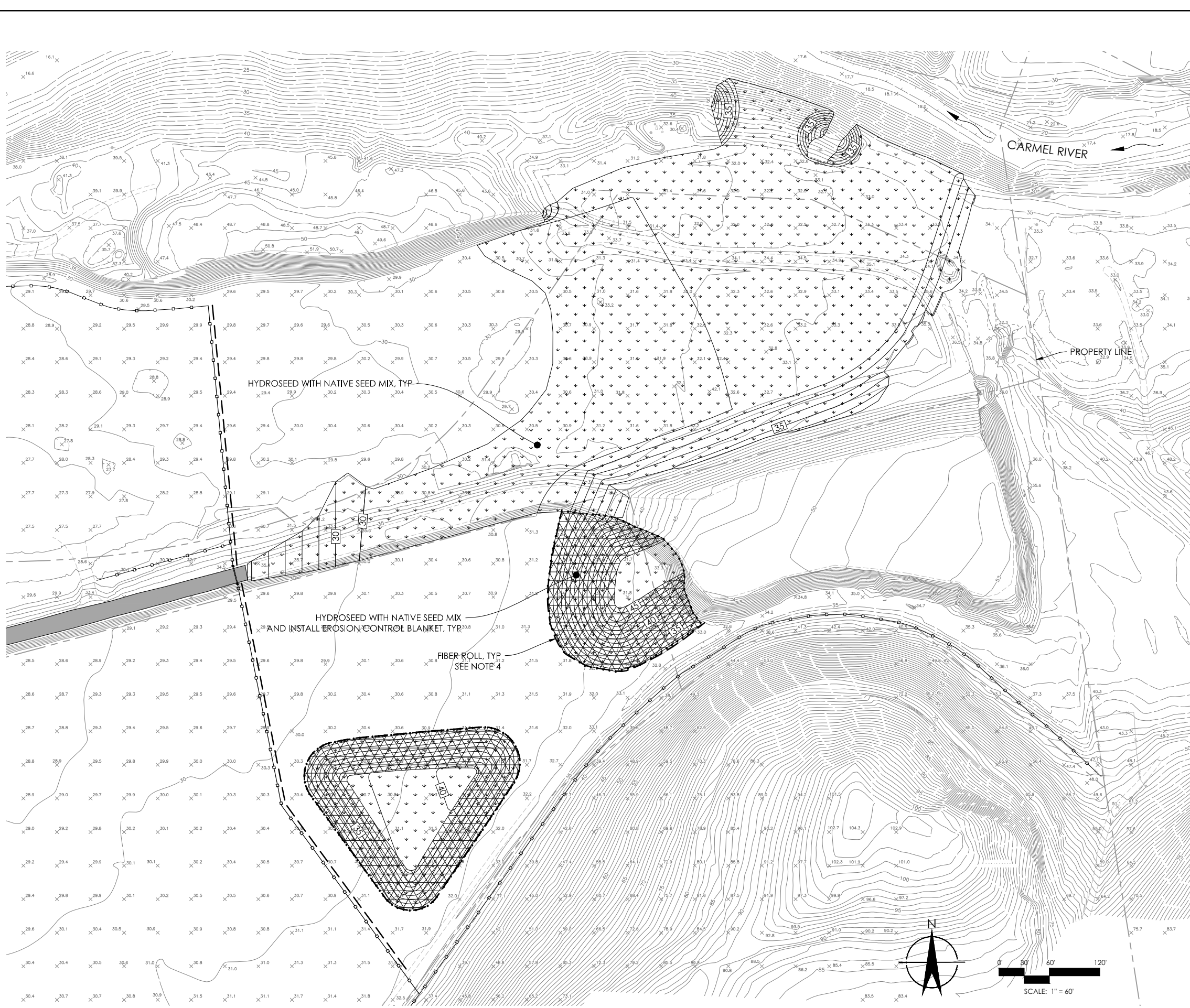
EROSION CONTROL PLAN 1" = 60'
