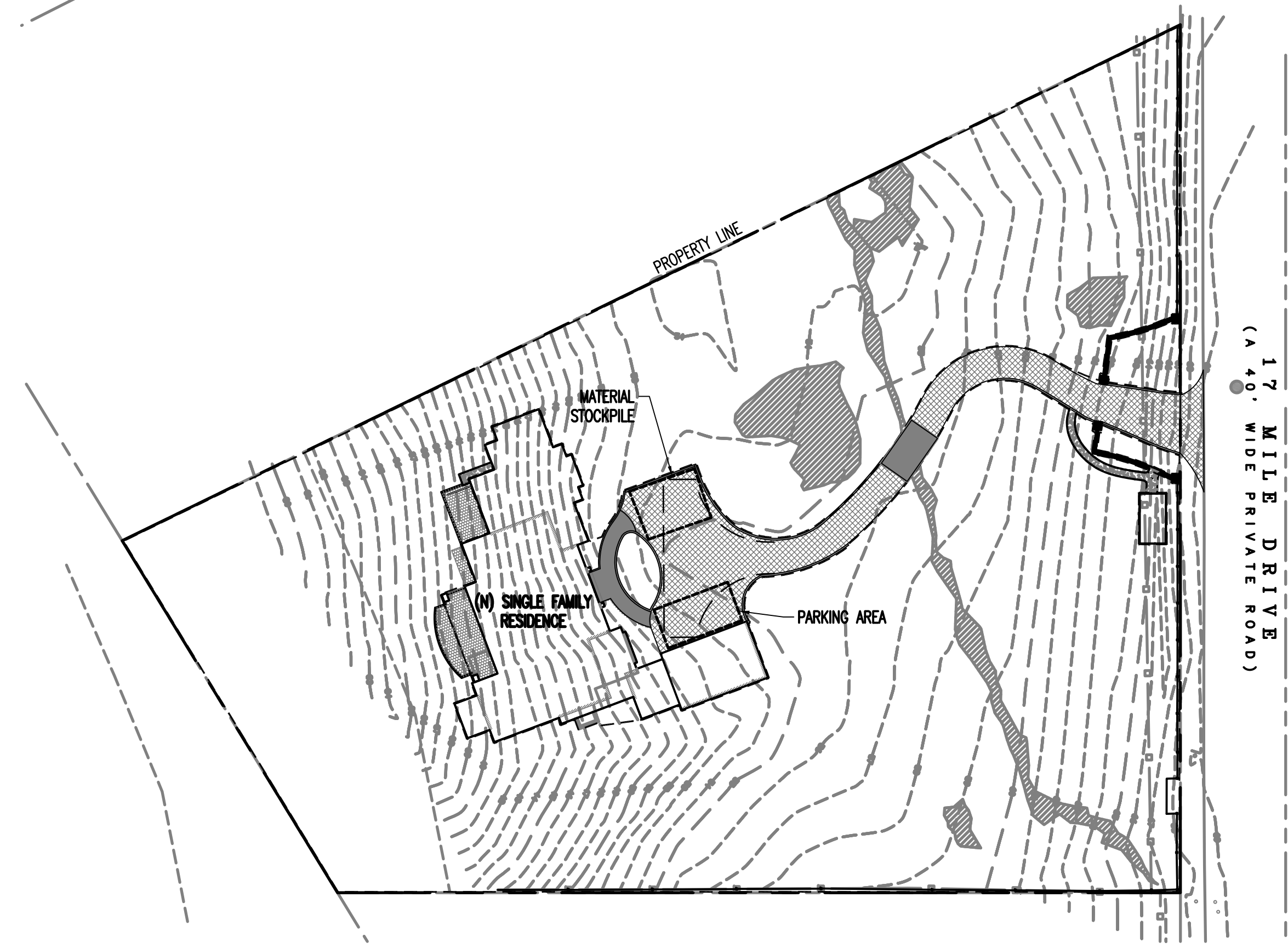
1 - EXCAVATION STAGING PLAN SCALE: 1"=40'
