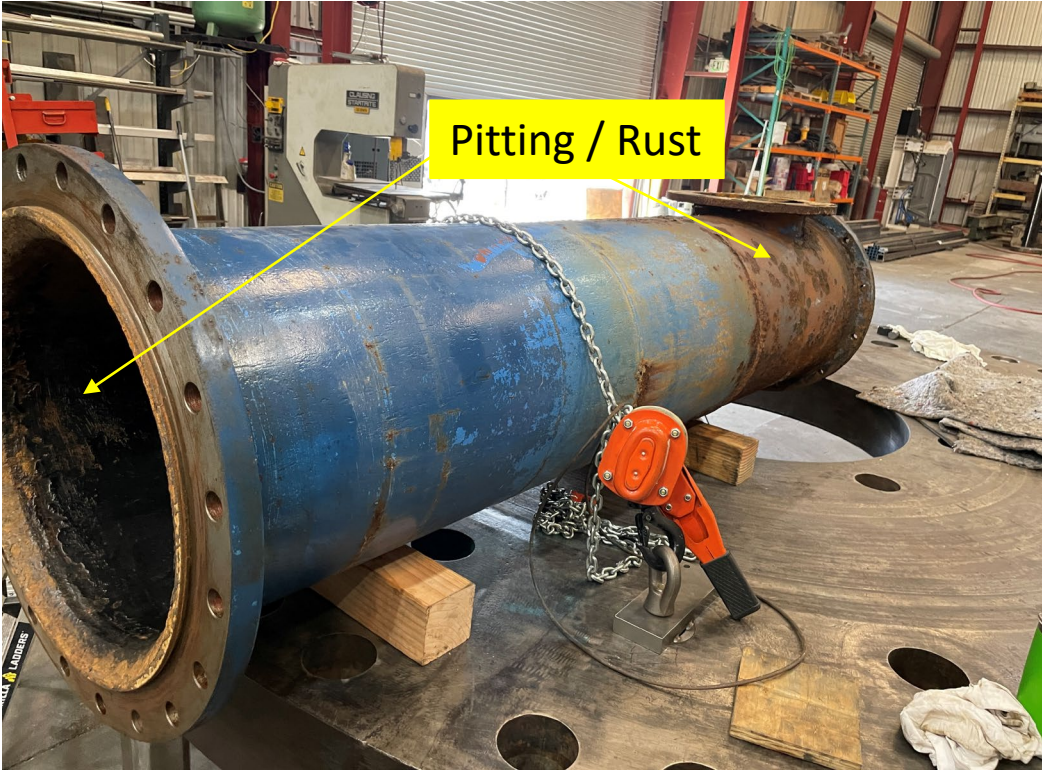
Turbine Column Housing
