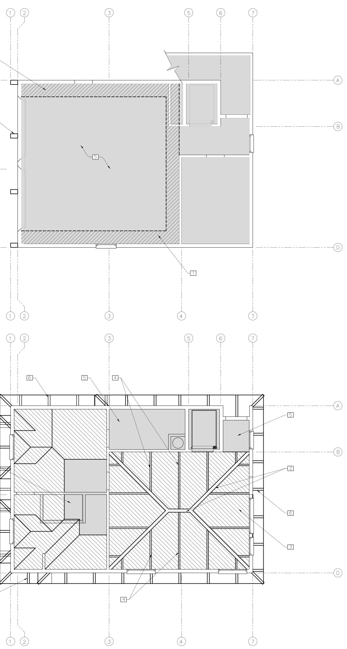
KEY NOTES SOFFIT SHOWN CROSS HATCHED 2 6X6 RD. WD. RAFTER STAINED 3 SLOPED OPEN BM. CEILING 4 3X4 RD. WD. BM. 5 FLAT CEILING 5/8-INCH TYPE "X" 6 4X8 RAFTER TAILS @ 48" O.C 7 DECORATIVE BM
