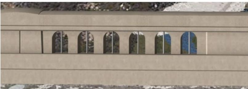
**Figure 1: Type 86-H Railing with 6 inch chamfered opening and 10 inch wide options.**
