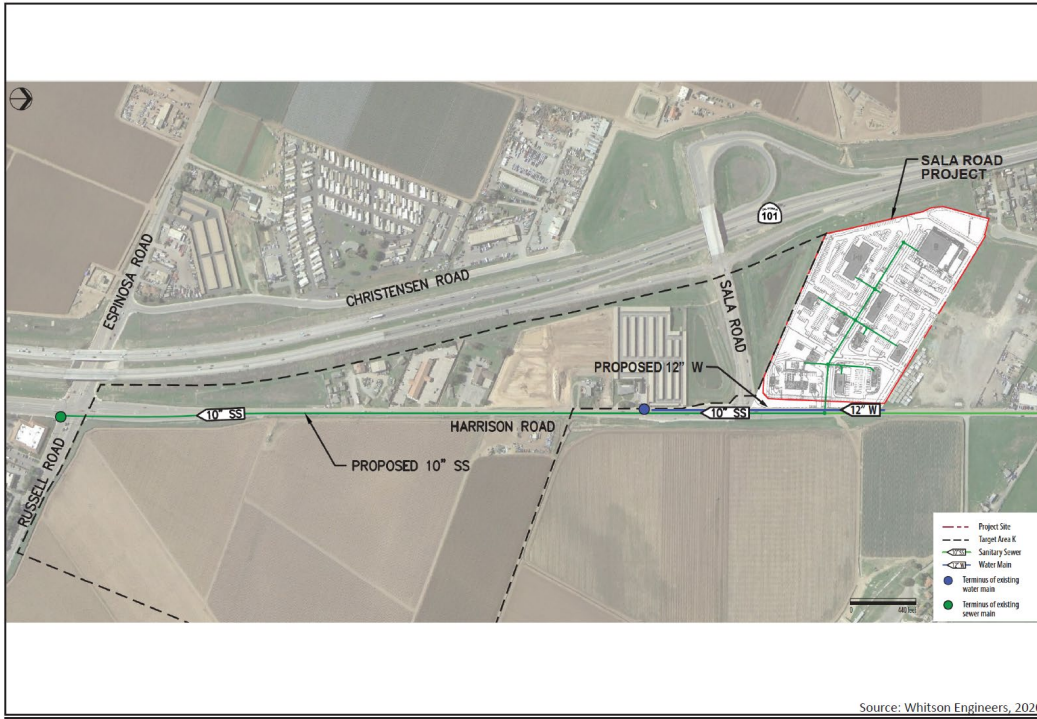
Off-Site Water and Sewer Infrastructure Improvements Sala Road Commercial Project Initial Study
