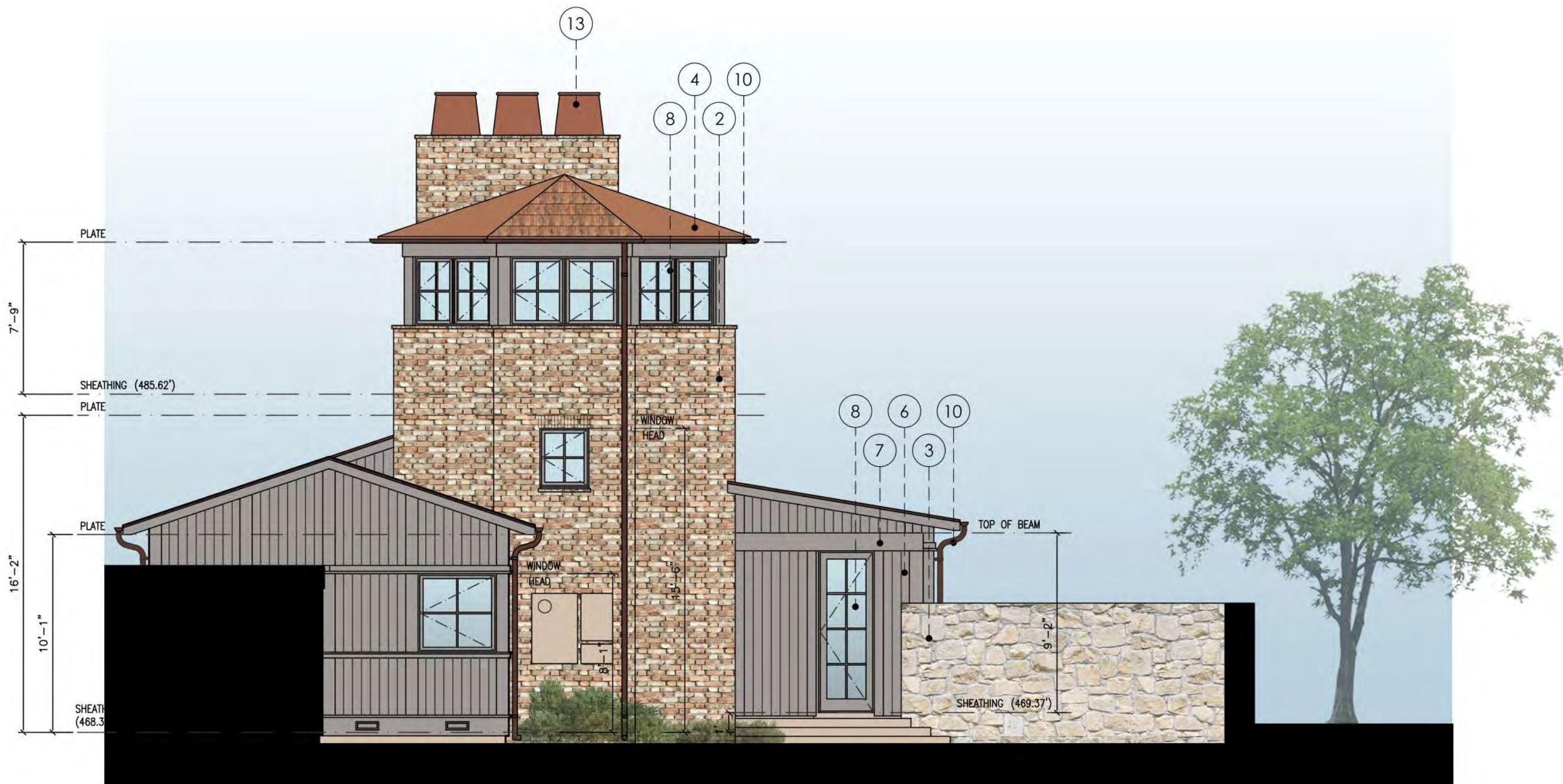
2 - SOUTH ELEVATION AT TOWER 3/16" = 1'-0"
