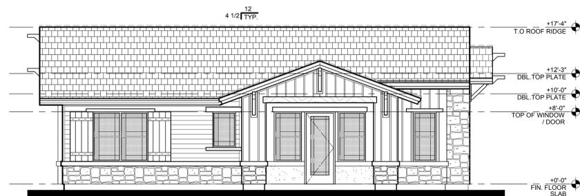
REAR ELEVATION - BUILDING TYPE 51 - B UNITS
