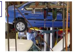
"Remove old in ground lifts, clean up, fill pits with reinforced concrete, and replace with above vehicle and equipment lifts. Secure Automotive Lift. Institute certified approved above ground lifts to replace five in-ground lifts in Light Repair Shop, two in-ground lifts in Service Station, and one in-ground lift at Toro Repair Shop."
