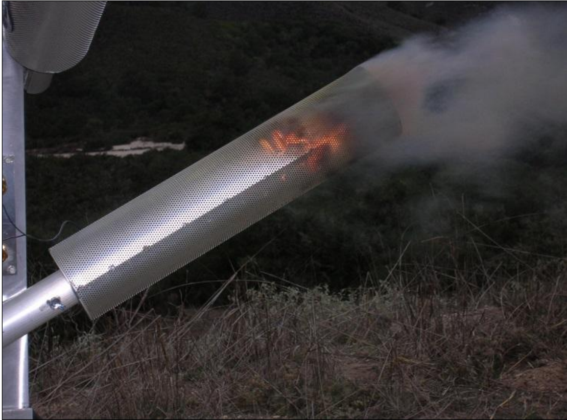
Figure 5.7 Flare Burning Inside Spark Arrestor
